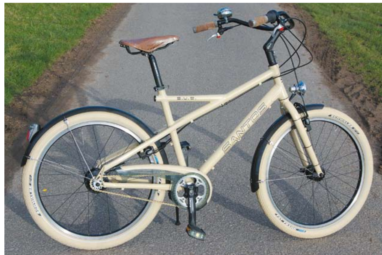
FAR LEFT: There's a Tubus-built rear rack option. LEFT: With flat bars the Santos has a very different look – and a more sporty and solid feel. RIGHT: Over-long cables and the upside-down brake levers are our fault; a factory flat bar install would be much neater.
