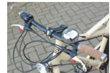
FAR LEFT: There's a Tubus-built rear rack option. LEFT: With flat bars the Santos has a very different look – and a more sporty and solid feel. RIGHT: Over-long cables and the upside-down brake levers are our fault; a factory flat bar install would be much neater.
